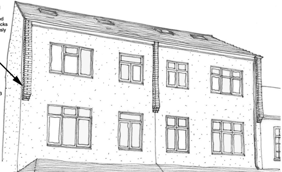
Figure 12 above:- existing party wall parapet not removed All new extensions with a parapet should match the existing next door parapets in materials and detailing.
