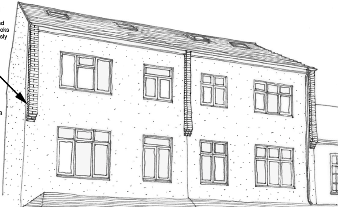
Above:- existing party wall parapet not removed All new extensions with a parapet should match the existing next door parapets in materials and detailing.
