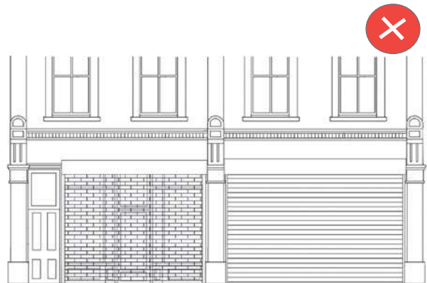
Picture 66. External Roller shutters are not appropriate.
