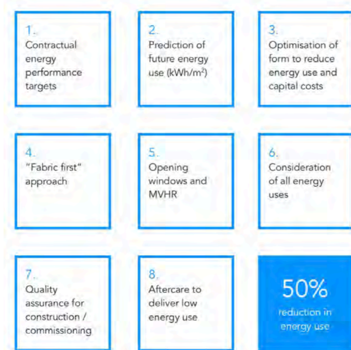
Figure 9 - Recurring features of a low energy building
