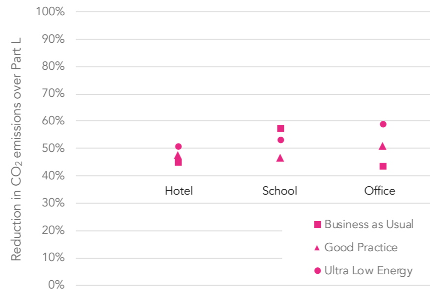
Figure 59 - Improvement in CO 2 emissions over Part L of the 3 fabric and ventilation cases for the three typologies (i.e. Hotel, School, Office)
